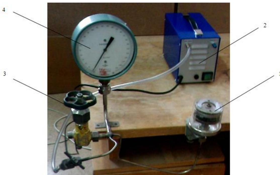
**Figure 12 – The device to determine the bubble point in filtering membrane elements (1 –cell, 2 – air pressure control unit, 3 – valve, 4 – pressure gauge)**
